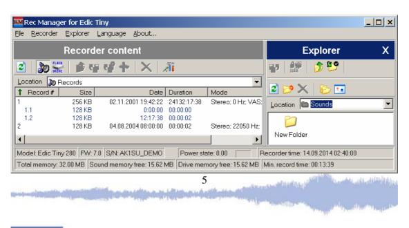
The program checks all parameters that are reflected on the Status Line. If the program detects that its version is incompatible with the recorder's EEPROM, the program shows a message that suggests renewing either the program or the EEPROM. To renew the program, first, the old program has to be removed. Then a new program should be installed. To renew the EEPROM, a special program has to be used. This operation is described in the chapter EEPROM.
